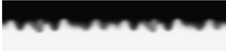
FIGURE 19. Plume structures at the early development of miscible Rayleigh–Taylor instability. Initially a layer of cold fluid (black) is on top of a layer of warm fluid (white), and a random perturbation is imposed at the interface.
